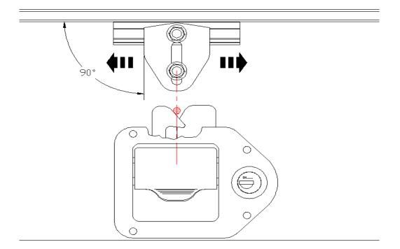
2) When the striker pin is correctly centered, tighten top bolt to set the location.
