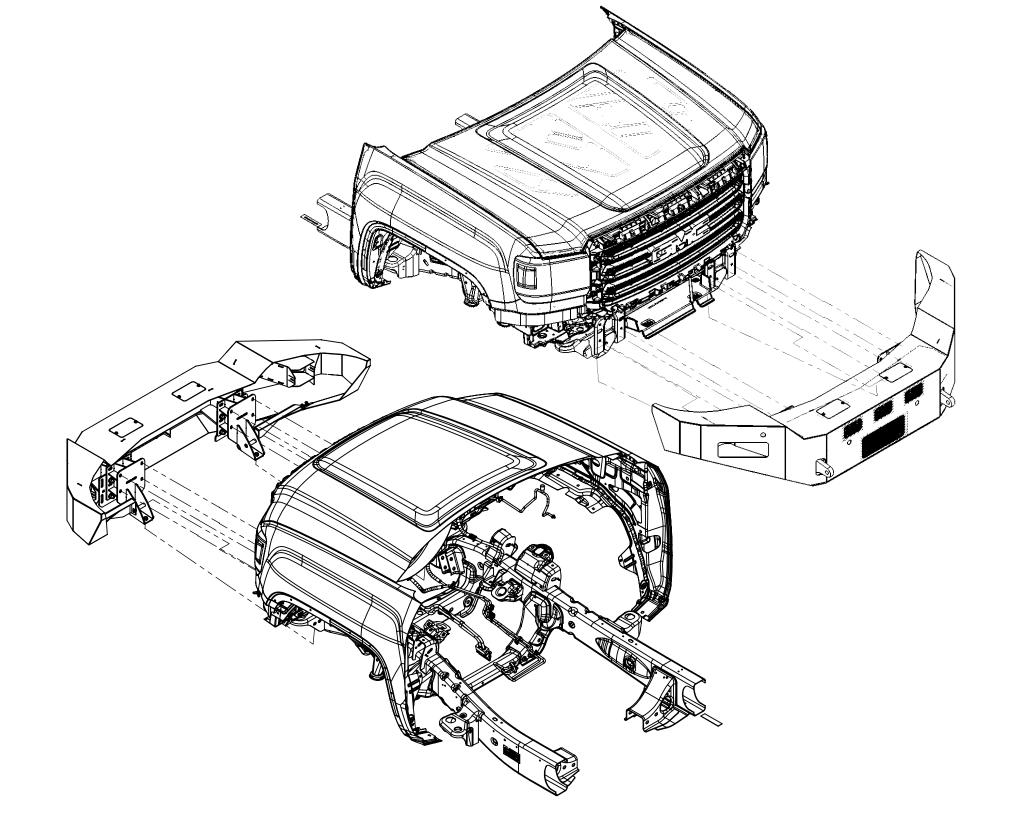
For some bumper applications, it will be necessary to tune the backup sensor housing to fit the new bumper. Most of the sensor housings utilize a plastic housing that snaps into the bumper. If the snap features do not work correctly, it will be necessary to file a small amount of the snap feature so that it snaps into the bumper correctly.
