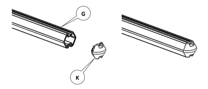
8 Slide the hex rails into the nuts from step 6.
