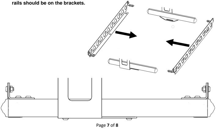
Drop in the decks (I) between the fences. If desired, one deck can be used instead of two. Ensure decks line up with slots in vehicle brackets and install bolts (M), washers (N), and nuts (O) into fences and through vehicle brackets to install. Center the rack and fully tighten all hardware at this time.
