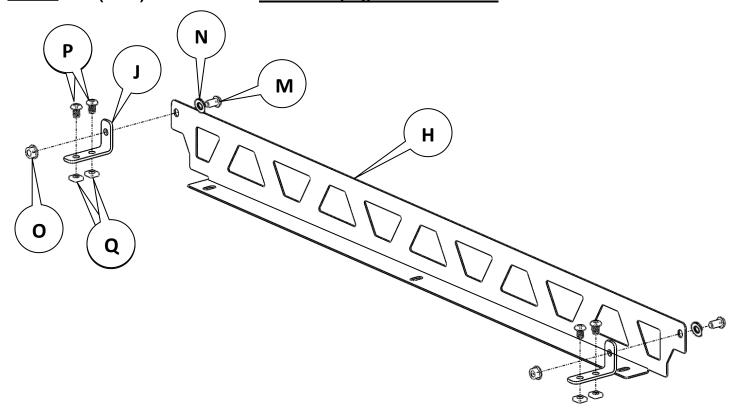
Slide the preassembled fences into the hex rails with the bends of the fences facing each other. The lower picture below is a side view of about where the fences and hex
