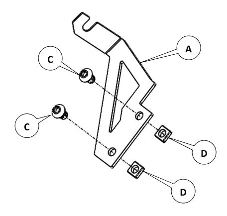
3 Slide bracket into A-Pillar channel and replace endcap. Fully tighten endcap at this time.
