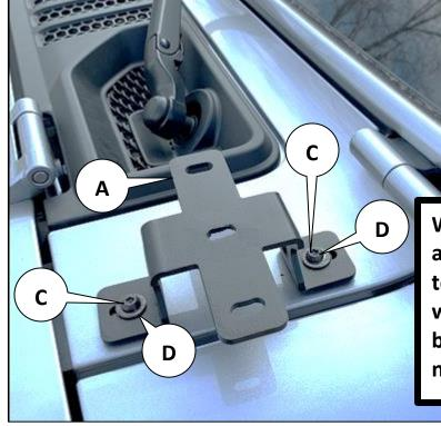
When bracket or any accessory is mounted on the top of the bracket the windshield will not be able to be folded down. Bracket is not intended for a Light Bar
