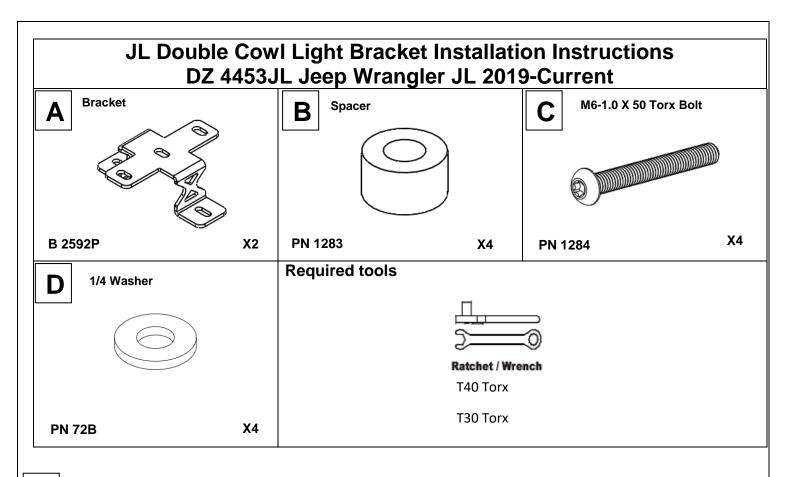
First remove the 2 upper bolts in the driver's side cowl using a T40 Torx.
