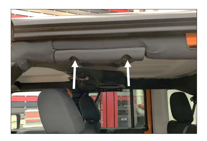
3 Install bolts (E), washers (F), and spacers (C) through the mounting bracket (B) and into the two mounting locations from the previous step. Fully tighten bolts at this time.
