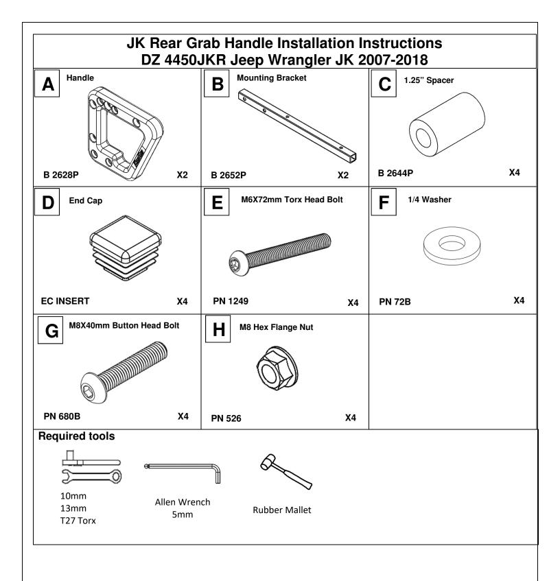
Install the end caps (D) into both ends of the mounting bracket (B).
