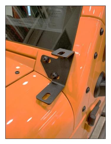
When Lower Light bracket is mounted the windshield will <u>not</u> be able to be folded down. Brackets A and B are not intended for a Light Bar.
