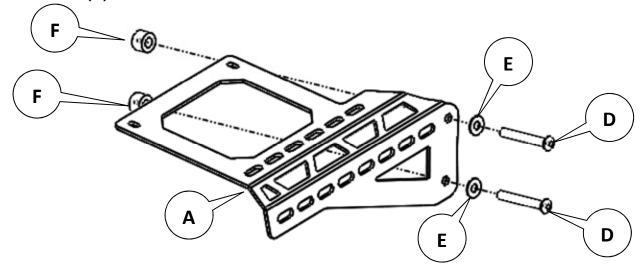
Install the bolts from the previous step into the lower holes of the cowl. <u>Do not fully tighten at this time.</u>
