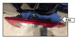
NOTE: The taillight may contain a blind spot sensor. Detaching the light and turning the ignition to "ON" may affect this sensor. Do NOT disconnect the taillight and turn the key.
