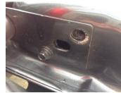
STEP 3) Using a 10mm wrench, loosen, but **DO NOT** remove, the lower bolt.
