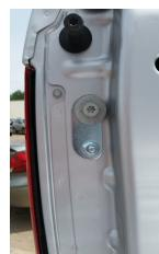
Tighten the bolt with the T50.
