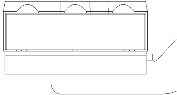
**Once the board is in the desired location, tighten the bolts that attach the board to the brace using a 7/16" wrench and socket.**
