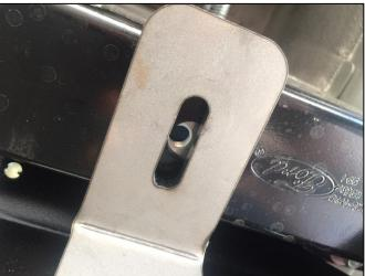
Insert bolt (F) and washer (J) into front mounting location. <u>Do not fully tighten at this time.</u>
