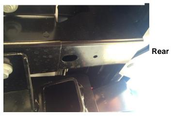
Insert the large thread plate (E) into the area shown below in the picture on the left.
