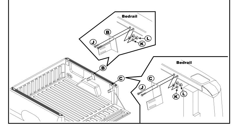
Place the wheel well toolbox (A) back into the vehicle truck bed inside of mounting brackets (B / C) as shown below. Use the existing holes in mounting brackets (B / C) as a guide to drill two 1/4" holes through the outside of the wheel well toolbox (A). <u>Note: See Steps 13 - 16 for mounting bracket (C) installation on</u> <u>1994 - Current Dodge Ram Pickup beds.</u>
