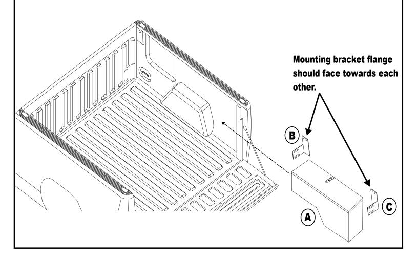
Remove the wheel well toolbox (A) from the vehicle bed and then use the marked hole locations as a guide to drill a 1/4" hole through the inside lip of the bed rail as shown below. <u>Note: See Step 13 - 16 for mounting bracket (C) installation on</u> 1994 - Current Dodge Ram Pickup beds.
