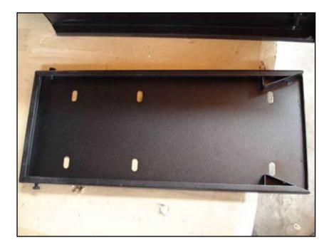
3. Position the mounting tray behind the fender flare of your choice, ensuring to have the front facing the tailgate.
