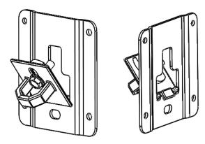
3. Align the threaded plate with the opening and push the tie down up against the bed mounting plate
