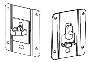
4. Move the bolt to the top of the slot and rotate the plate 90 degrees. Pull out on the tie down to keep the threaded plate under tension and tighten the bolt with a 13mm socket.
