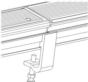
Note: Some trucks will have a center stake hole that will not allow the hold down clamp to bridge the joint of the main housing and bungee box. In this case, it is important to make sure that the two hold down clamps are installed on the front main housing and two hold down clamps are installed on the rear main housing (One as far forward as possible and one as far back as possible).
