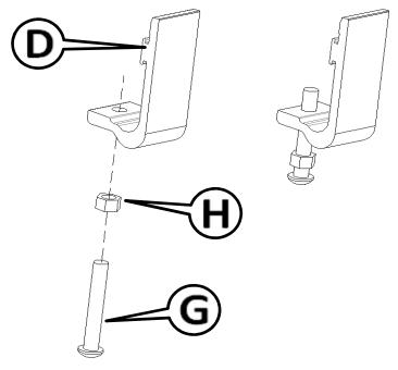
Slide the 4 hold down clamps into the bottom channel on the back side.
