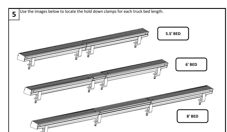
The end hold down clamps should be as close to the end as the truck bed allows, but still completely in the channel of the extrusion.
