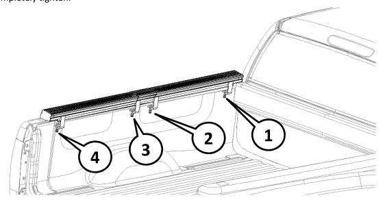
7 Once the 3/8" bolts have been tightened, using a 9/16" open end wrench, tighten the nut against the bottom of the hold down clamp.
