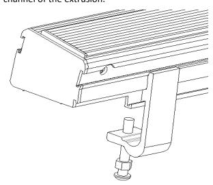
For applications with the bungee box, the hold down clamp needs to bridge the joint between the rack section and the bungee box equally.
