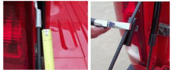
Failure to remove the limiter and to install the cable clip will cause the cable to bind or become caught between the shock and truck bed. This may lead to vehicle damage, so these steps MUST be done.
