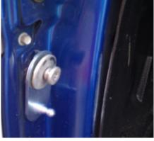
Tighten the bolt with the T45.
