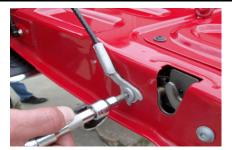
To remove the limiter, pry up one edge of the flat nut with a screwdriver. Hold this edge with a pair of pliers and spin the bolt out of it.
