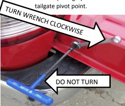
The nutsert should be tightened 9 360 degree turns.
