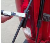
Failure to remove the limiter and to install the cable clip will cause the cable to bind or become caught between the shock and truck bed. This may lead to vehicle damage so these steps MUST be done.
