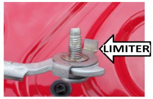
Once the limiter is removed, reinstall the cable mount to the tailgate.
