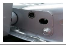
STEP 3) Using a 10mm wrench, loosen, but **DO NOT** remove, the lower bolt.
