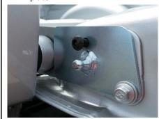
Tighten the button head with an M5 allen wrench and the other bolt with a 10mm wrench.
