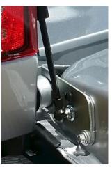
Install the cable back onto the cable bolt, and the larger part of the shock on the ball mount.
