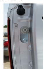
Tighten the bolt with the T50.
