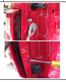
Inside the taillight opening , use an 11mm socket to remove the 2 nuts holding the rubber block in place.
