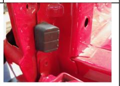
After removing the rubber block reinstall the taillight. If the rubber block is not removed, it will interfere with the shock.
