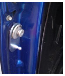
Tighten the bolt with the T50.
