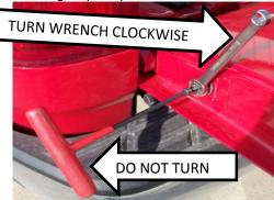
The nutsert should be tightened 9 360 degree turns.
