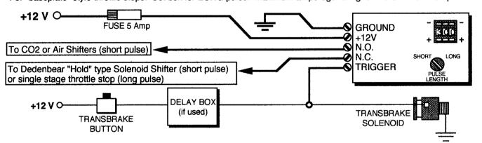
Typical wiring diagram for NITROUS OXIDE systems: Set box for LONG pulse.
