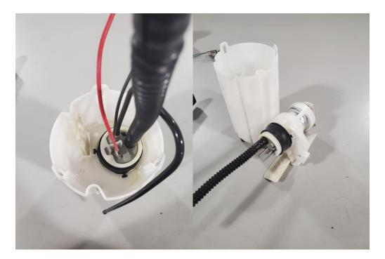
4 – Remove the pump, pre-filter sock and plastic pump retaining pieces from the pump assembly, you will be reusing the rubber portion and the larger outside plastic portion. (See Picture)
