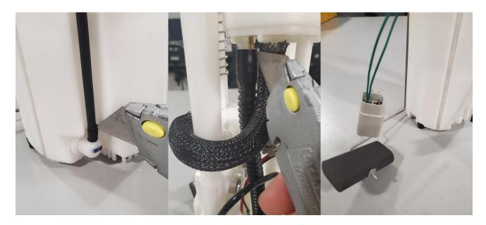
2 – Separate the bucket from the center section by unlatching the clips around the edge of the bucket. Slide the module apart.
