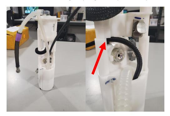
8 – Remove the flare off the very end of the venturi hose, and slip on the 6.1mm hose clamp, heat the hose and install it over the factory venturi jet inlet nipple, this can be difficult due to the angle and size of the parts in question.
