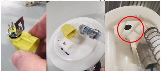
12 – The factory fuel pump power and ground wires can be removed or covered so they will not short on the module. Attach the supplied Brushless pump harness to the bulkhead and the DW440 pump. Re-attach and connect the fuel level sending unit wiring and sensor to the module.
