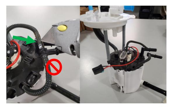
2 – Separate the bucket from the center section by unlatching the four clips around the edge of the bucket.
