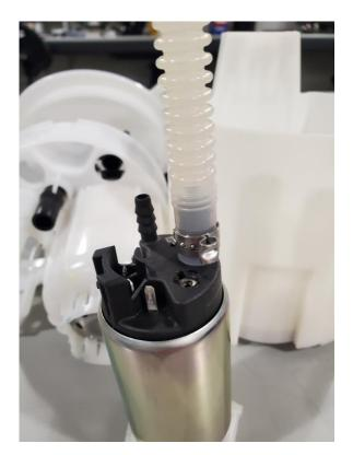
6 – Attach the supplied 1/8" venturi hose to the venturi jet inlet on the bucket and clamp with the 6.1mm clamp. Install the center section into the bucket. Make sure to snap the venturi jet assembly back into place.
