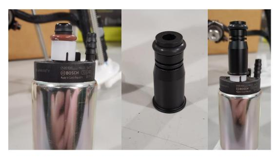
6 – Insert the pump into the center section, lubricate the O-ring to aid installation, the outlet extension should be fully seated into the center section. It is also necessary to install the wiring harness currently and fish it through the opening for the OEM harness.
