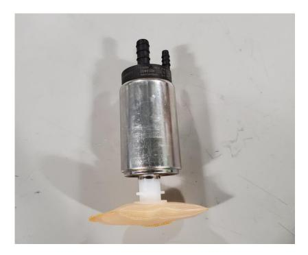
6 – Install the pump into the bucket and slide the plastic pump outlet adapter onto the outlet of the DW440 pump and the nipple from the bucket. The DW440 has a larger barb than the OEM Ford pump, be sure to use the supplied lube to ease install. Once the pump outlet is seated on the pump and the module, reinstall the 2 screws that hold it in place, and the 3 that hold the lid onto the bucket.
