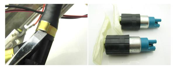
3 – use a flat head to gently pry this opening to allow clearance for the two (2) supplied DW 2 1/4" hose clamps
