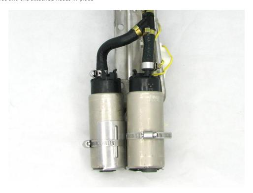
6 – install the fuel socks onto the bottoms of the DW400s
