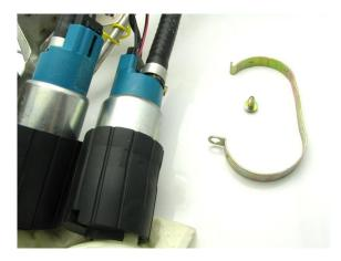
2 – loosen the OE hose clamps from both pumps and remove the pumps. Remove the upper hose clamps and remove the OE hose (it may need to be cut to remove, careful to not score the barbs underneath). Install the supplied DW hose, the longer hose goes on to the angled inlet
