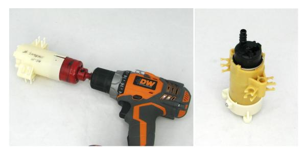
4 – trim the pump subassembly base to fit around the inlet of the DW400. Temporarily install the screws to hold the base to the subassembly
