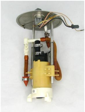
6 – trim the hook on the fuel level sender and then install the fuel level sender onto the pump subassembly. Tighten the subassembly bottom cap screws and install the pump pre-filter
