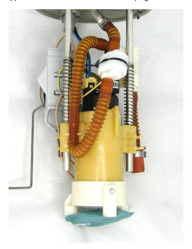
8 – reinstall the assembly into the fuel tank and attach a length of hose to the outlet of the pump assembly allowing it to drain into a fuel safe container and prime the fuel pump assembly
