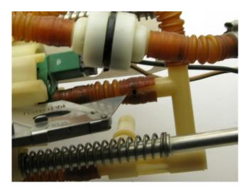
2 – disconnect the fuel level sender from the electrical harness and remove the pump assembly with springs and set aside, DO NOT cut the remaining OE tubing!
