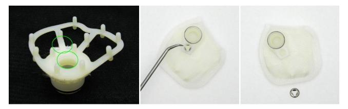
6 – follow step 6 if the supplied high-pressure PRV will be used. Remove the white retainer clip and gently pry the OE PRV from the filter assembly. Using the supplied Superlube, lube the oring on the HP PRV and press into the filter assembly. Reinstall the PRV retainer clip
