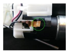
3 – lift up on the four (x4, green circle) tabs holding the white cap onto the black housing and pull the cap away from the housing enough to insert a flat screwdriver in to depress the electrical connector to the pumps in and gently pry up
