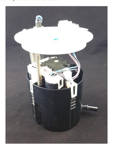
10 – reinstall the assembly into the fuel tank and attach a length of hose to the outlet of the pump assembly allowing it to drain into a fuel safe container and prime the fuel pump assembly
