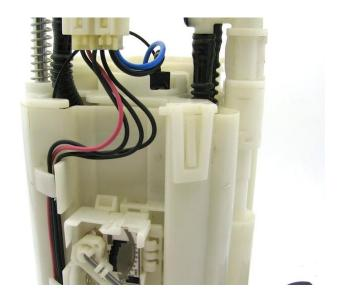
1 – disconnect the connector for the fuel level sender and depress the tabs (black) to separate the bucket from the assembly
