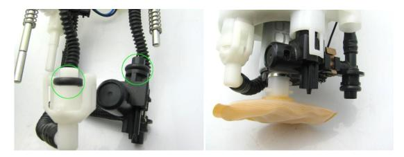
8 – Install the bucket assembly onto the center section
