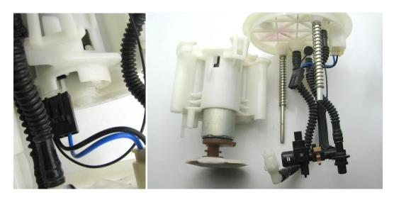
4 – remove the fuel pump from the center section by using 2 flat-head screwdrivers to open the retaining tabs (green)
