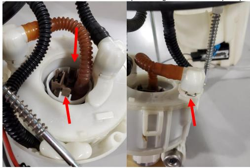
4 – Remove the factory fuel pump from the center section, once removed gently remove the filter feed adapter from the factory convoluted hose, this can be done by slicing the OEM hose with a knife, take care not to damage the plastic fitting under the hose.
