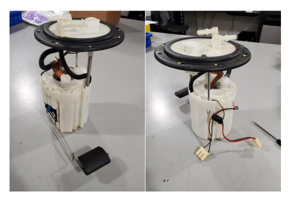
2 – Lift the locking tabs that hold the top hat support rod in place. Unlock the venter section by lifting the three locking tabs around the top of the bucket. Separate the bucket from the center section by lifting.
