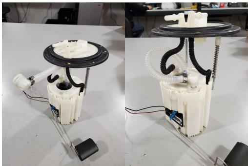
8 – Install the supplied pump wiring adapter and reattach the fuel level sending unit wiring.
