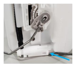
2 – Unplug the factory electrical connectors for the pump and sending unit, unclip the wires from their holders on the filter center assembly.
