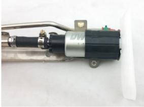
5 – install the pump retaining strap
