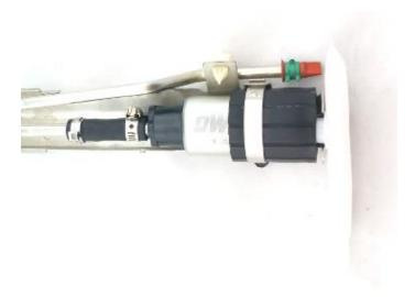
6 – reinstall the assembly into the fuel tank and attach a length of hose to the outlet of the pump assembly allowing it to drain into a fuel safe container and prime the fuel pump assembly
