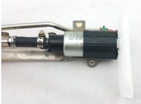
5 – install the pump retaining strap
