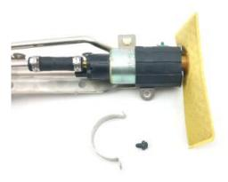
2 – loosen the OE hose clamp from the pump outlet side of the hose and remove the pump, if the OE hose is in useable condition, the other permanent clamp may be left in place. If the hose needs to be replaced, remove the second permanent clamp and remove the hose
