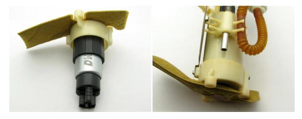
5 – install the hose and clamps onto the pump outlet and connect the hose to the assembly, the hose may need to be cut to length. Plug in the OE electrical connector
