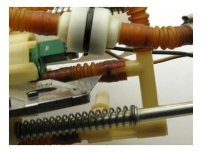
2 - remove the 2 screws (3/16" head) from the base and pull out the fuel pump
