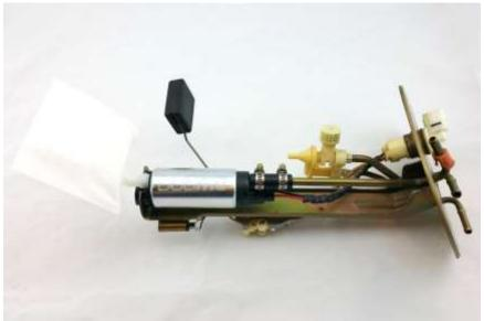
4 – reinstall the assembly into the fuel tank and attach a length of hose to the outlet of the pump assembly allowing it to drain into a fuel safe container and prime the fuel pump assembly
