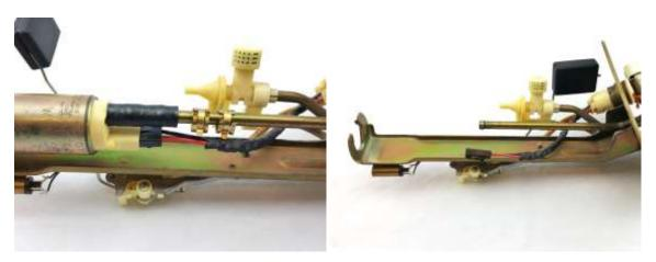
2 – prep the DW300 by installing the fuel sock and retainer. Start installation of the retainer by pressing it on with your thumb, then use a 4-5mm deep socket to press it on the rest of the way
