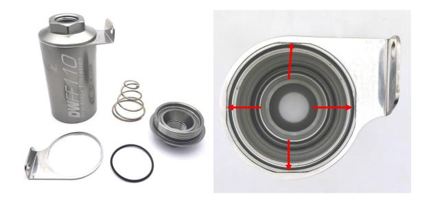
5 – Both caps should be torqued to 15-20lbs using an 1-5/16" or 34mm aluminum wrench. The pre-installed O-rings are what seals the housing, DO NOT OVERTIGHTEN!
