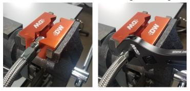
Make sure the nut is well secured and tight. Lining up the hex on the nut and the hose end is a nice touch, as later on in the vehicle it makes for sliding on a wrench that much easier. The picture below it what the finished product should look like. As with all fuel system components, double check for any leaks before driving the vehicle.
