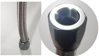
**4** Place some grease on the fitting on the hose end before threading it into the nut. This will prevent it from biting the hose and tearing it.
