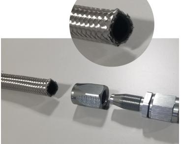
**3** Take the nut and start to slide it onto the hose. There should be no frays that stick out. That will keep the nut from going on properly. Once the nut has begun to go over the hose it will take a bit of force to get it the rest of the way securely. In the picture below I used the table by placing the nut face down and pushing the hose downward. 2<sup>nd</sup> picture you can see where the hose should be firmly seated at the bottom of the threads.
