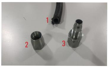
**1 – CPE Hose** is available in black nylon braided (shown) and bright stainless braided. The DW CPE (Chlorinated Polyethylene) hose is made of a synthetic rubber with has a pressure rating of 500 psi and a temperature rating of -40 to 300 Degrees Fahrenheit. It is compatible with Pump gas, most race fuels, and E85.
