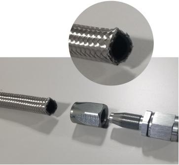
**3** Take the nut and start to slide it onto the hose. There should be no frays that stick out. That will keep the nut from going on properly. Once the nut has begun to go over the hose it will take a bit of force to get it the rest of the way securely. In the picture below I used the table by placing the nut face down and pushing the hose downward. 2<sup>nd</sup> picture you can see where the hose should be firmly seated at the bottom of the threads.
