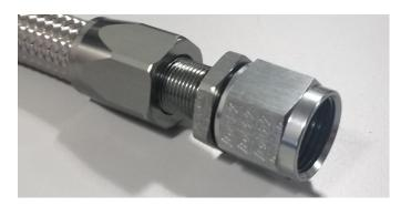
**6** After getting the threads started it makes it easy to use a vice with our Soft Jaws (6-02-1007) for AN hoses. If you don't have them using an AN wrench works as well. Place the hose end and tighten the hose end nut with a AN wrench to not damage the fitting.
