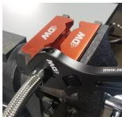
Make sure the nut is well secured and tight. Lining up the hex on the nut and the hose end is a nice touch, as later on in the vehicle it makes for sliding on a wrench that much easier. The picture below it what the finished product should look like. As with all fuel system components, double check for any leaks before driving the vehicle.
