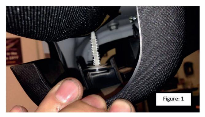
3. Moving on to the A-pillar, with the Phillips screw driver remove the center of the push pin that retains the factory A-pillar. **TIP:** The treads on the center pin, are not very strong. Use light pressure when unscrewing the center pin. Once it is out far enough to grab with the needle nose pliers, switch tools, and remove the whole assembly (Figure: 2).
