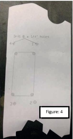
12. With the 1/16" bit drill hole #1. Use caution when drilling holes on the curve. The drill bit may try to walk, if it does a poor installation may result.
