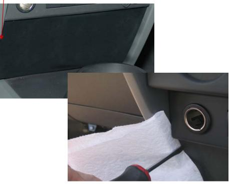
3. Push screw driver to the side to release the clips. Pull back the panel with your hand and remove panel.
