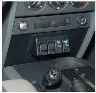
9. Install the 2 clips on to the switch panel by pushing down on the clips with your hand.
