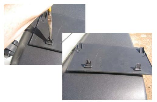
5. With the needle nose pliers compress the clips flat so they will clip on the Daystar switch panel.
