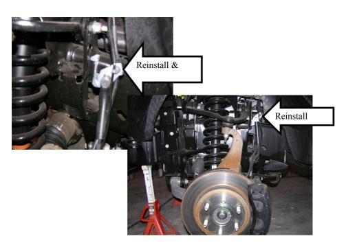
13. Tighten the lower strut bolt and nut.
