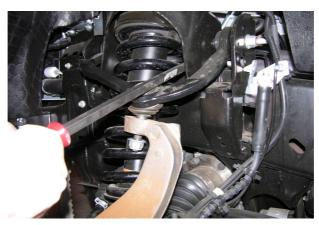
11. With the ball joint nut installed on the ball joint tighten the upper strut nuts .
