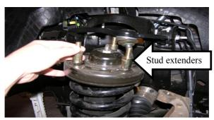
8. Install the spacer lift on top of the strut plate.
