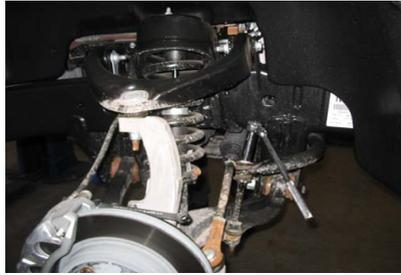
7. Remove the lower strut bolt and nut.
