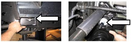
5. Place the floor jack under the Jeep tub between the front and rear wheel. Rise up the jack with the 2x4 jacking block on top of the jack and remove only one side at a time of the bolt and nuts from the Jeep mounts.
