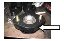
9. With the spacer mount installed. Install the mount into the fame support. **NOTICE: When** installing the front grill mount put the 2 studs in grill frame first, using the 2 studs and nut to hold the mount in the grill.
