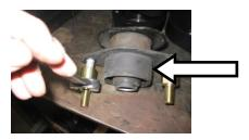
8. With the extenders tight install the body mount spacer over the stock mount.
