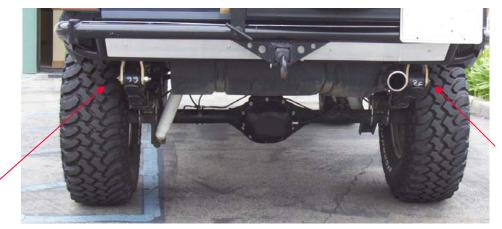
22. With all four tire and wheels on the ground check the lug nuts. Torque to factory spec.
