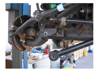
4. With the track bar disconnected install the track bar drop down bracket (S10921) and mark the hole in the axle bracket that need to be drilled.
