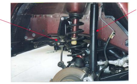
3. Disconnect the track bar from the axle side on the passenger side .
