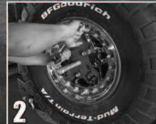
2 Install the new stud extensions, bolt on the plate.
