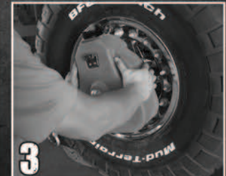
3 Install Cam Can. Cams lock it in securely and the shaft holds all the weight safely.
