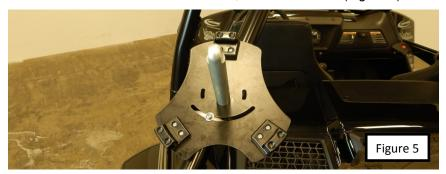
10. Install your Cam Can on to the plate, and you are finished!
